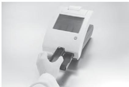
Remove the test cassette from the foil package and place the cassette on the test table.
