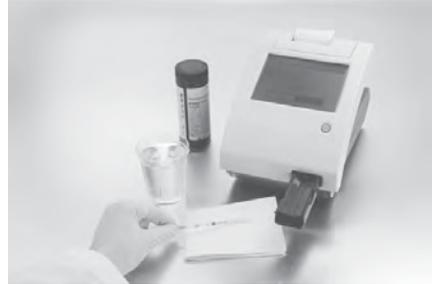
**4** Place the reagent strip in the channel of the table with the test pads facing up. Slide strip to end of the channel.
