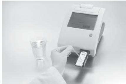
At the end of the 8 second countdown, the test table and cassette will automatically be pulled into the instrument.
