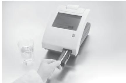
**NOTE:** A warning message displays if you are not using a Siemens reagent strip. Press **OK** to continue. The Results may not display if you are using a non-Siemens reagent strip. Repeat the test using a Siemens reagent strip.
