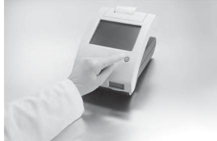
This is the first screen displayed. The analyzer will run an automatic system diagnostic test each time it is turned on.
