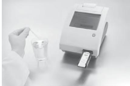
**2** Add entire contents of the pipette into the sample well of the test cassette.
