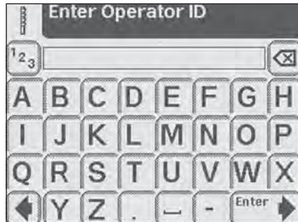
Use the keyboards to enter Operator Name using a maximum of 13 characters. Touch **Enter** when you have finished entering the Name and to move to the next screen.
